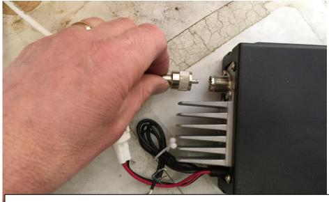
Connect aerial coaxial connector and hand tighten
