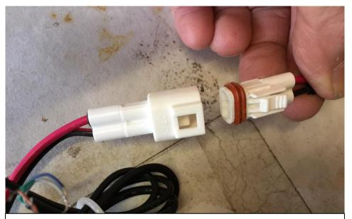
Push together power leads. To remove, push clip in and pull apart
